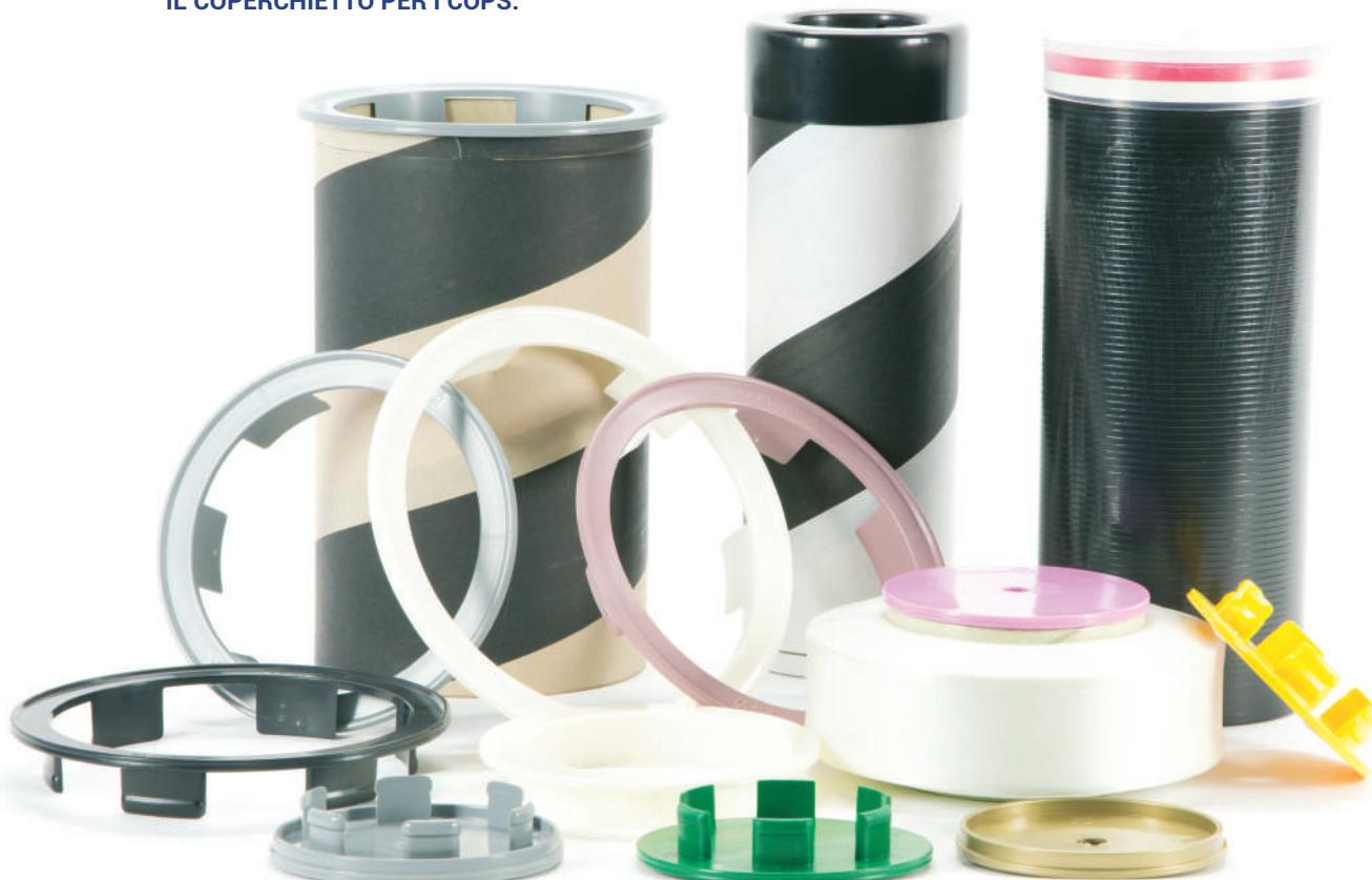
*The unwinding caps is used as protection for board of the paper tube and of the plastic tube on hosiery machines, the caps help the unwinding of yarn and avoid the breach of it. There are many types of caps with many different measures for different types of tubes.*
